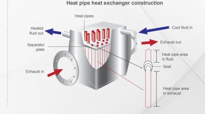
Heat pipes are sealed vacuum tubes containing a small amount of fluid that conducts heat from one end of the tube in a hot exhaust gas stream to the other end placed in the water or gas to be heated. Heat transfer is near instantaneous and highly efficient, with no cold spots and little thermal stress along the pipe's length for long, reliable life
