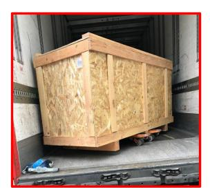
The unacceptable examples above show poor pallet and vehicle load, which makes it a dangerous delivery.
