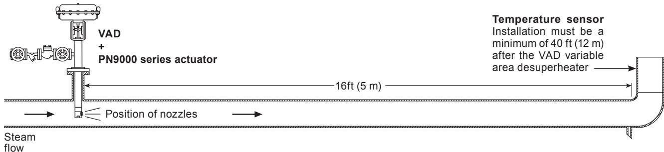
The **temperature sensor** should be located a minimum distance of 40 ft (12 m) after the VAD, however for optimum temperature control it is recommended that it be installed at the point of use.
