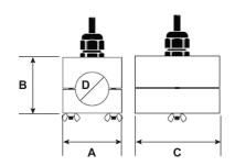
Fixed Small Pipe U-Bolt Connections CF, CL ANSI/ON and Copper 2" Models /Not for metric pipes.)
