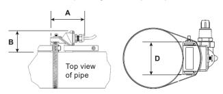
NZ, WZ, HZ, LZ, YZ Pipes Larger than 2" (51 mm)
