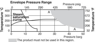
\*PMO Maximum operating pressure recommended. A - A Flanged ANSI 300, screwed and socket weld C - C Flanged ANSI 150
