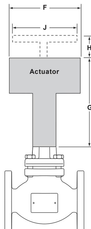
**Dimensions/weights** for the **EL and AEL actuator ranges** approximate in mm and kgs (inches and lbs)
