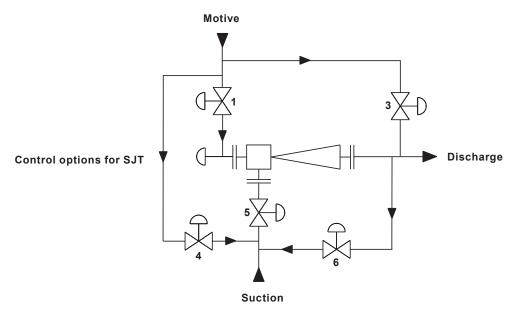
**Note**: You cannot choose Options 1 or 2 if the SJT Steam Jet Thermocompressor is 'Sonic' Most applications will only use one of the options. Some applications do not require any control. An SJT Steam Jet Thermocompressor will always balance itself to the system pressures.
