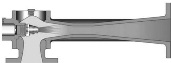
Fig. 3 Cross section of fixed nozzle type SJT Fixed Orifice (loads stable, less than 10% variation)
