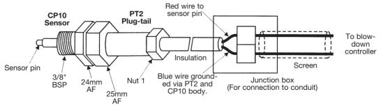
The supply to the Sensor and Plug-tail must be provided by a low voltage limited power source. Spirax Sarco Blowdown controllers provide this type of supply.
