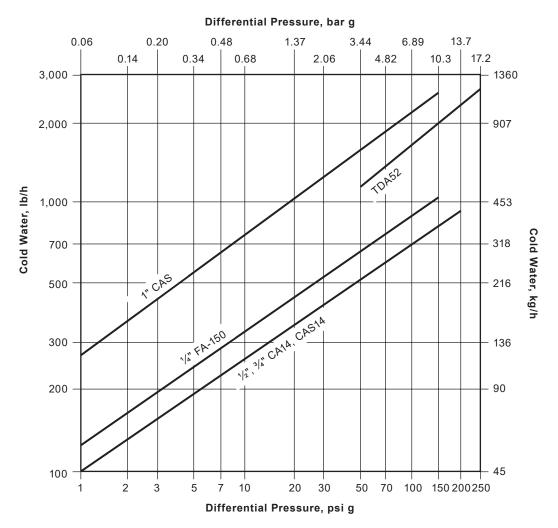
Cold water capacity for single-phase flow of liquids with a specific gravity of 1.0
