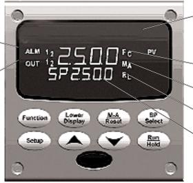
Upper display with 4 larger digits shows process Variable value (normal operation) or parameter value (configuration). Selectable decimal position.
