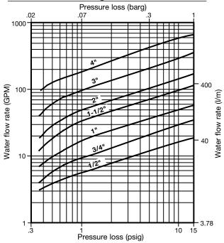
Pressure loss diagram with open valve at 68°F (20°C).
