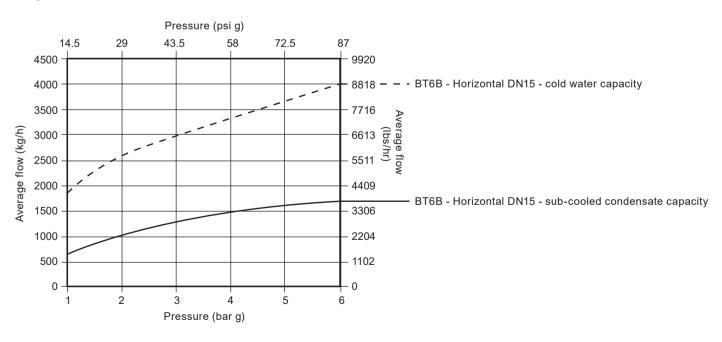
**BT6B Horizontal Sanitary Balanced Pressure Thermostatic Steam Trap**
