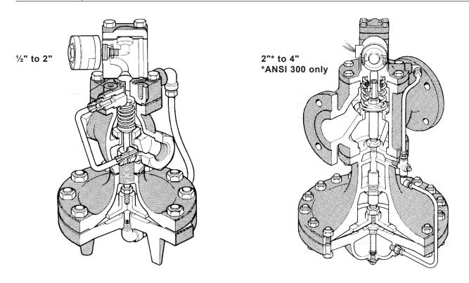
Typical applications On/Off control of steam flow in response to remote manual or automatic electrical signals which may originate at safety switches, timers, manual switches, etc.
