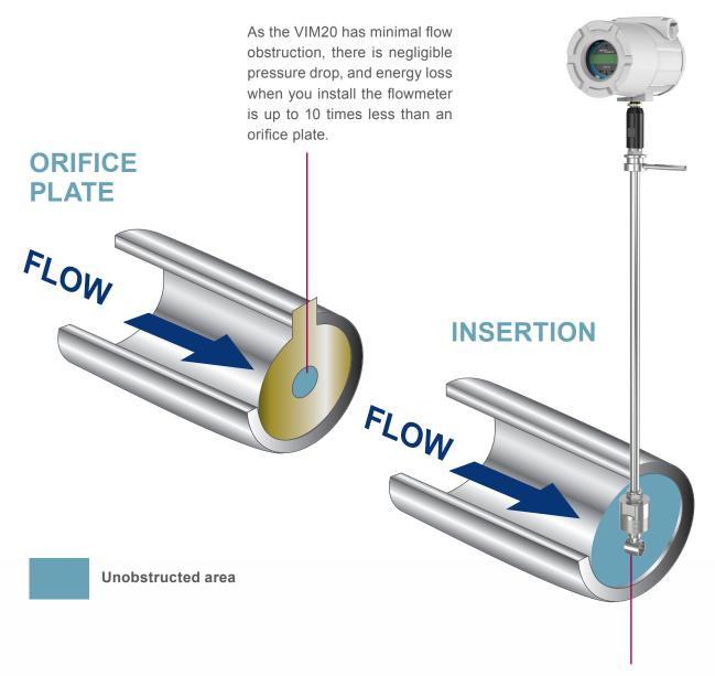
The insertion probe occupies a small area, leaving most of the pipeline unobstructed. Because it has a low pressure drop it is very efficient and flow pressure remains high.
