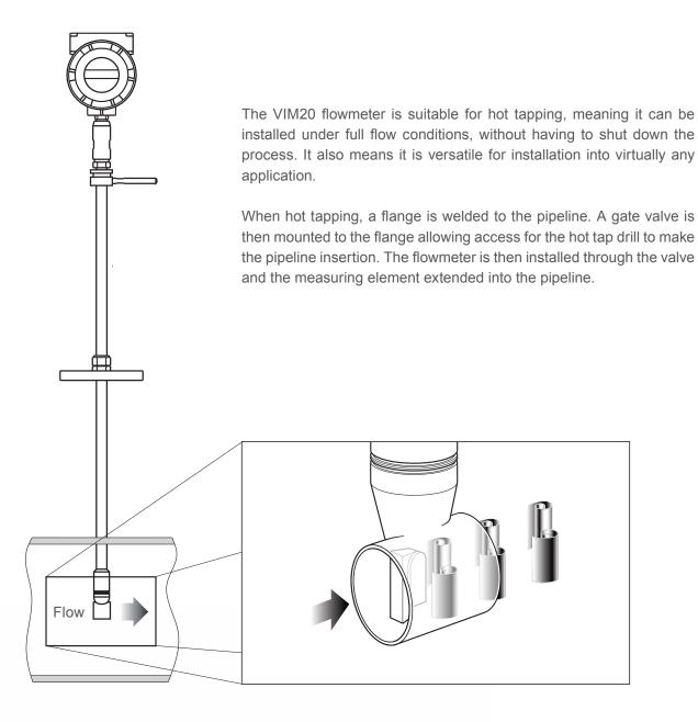
As the VIM20 can be fitted directly into operational pipework, installation is quick and easy without process shutdown. The cost of labor is reduced and data can be gathered more swiftly. Typical savings can be as much as 80% for DN600 (36") pipelines and 50% for the DN250 (10") pipelines.
