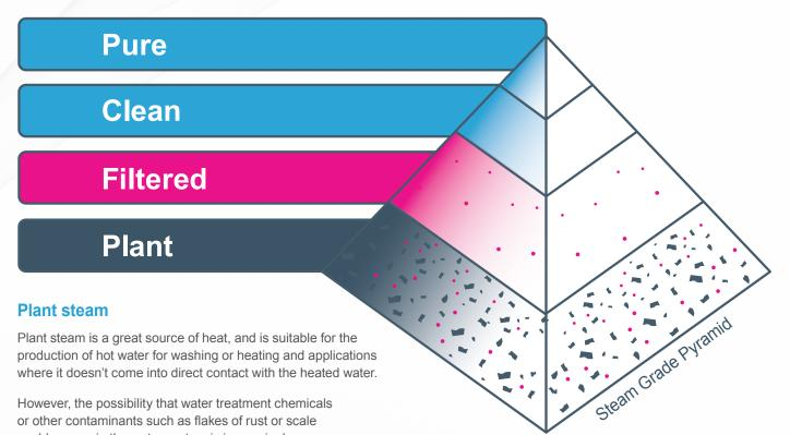
Plant steam is a great source of heat, and is suitable for the production of hot water for washing or heating and applications where it doesn't come into direct contact with the heated water.
