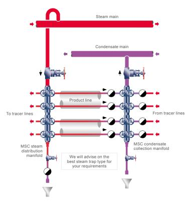
construction insulation can be awkward because of their widely differing geometry. However, our forged MSC series manifold are pre-assembled, minimizing the need for on-site fabrication and testing.
