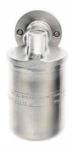
The UIB30 and UIB30H are sealed inverted bucket steam traps for either horizontal or vertical installation. Designed for higher capacities, when installed with a suitable pipeline connector, the UIB can easily and simply be removed without breaking into the pipeline, thus reducing system downtime.
