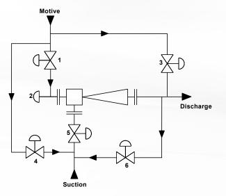
Most applications will only use one of the options. Some applications do not require any control. A Steam Jet Thermocompressor will always balance itself to the system pressures.
