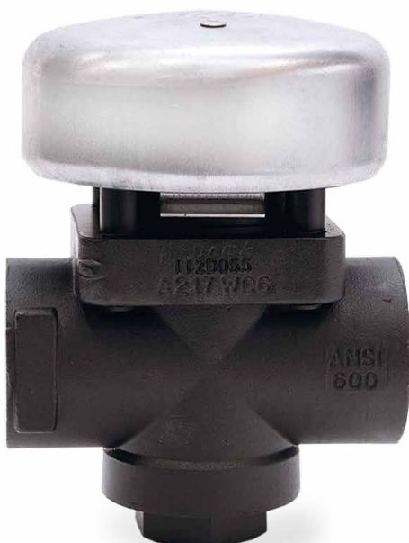
The TD62LM and TD62M have an integral strainer and a replaceable seat. They have been specifically designed for mains drainage applications up to 62 bar g. The TD62LM is suitable for relatively small condensate loads on superheat and mains drainage applications. An insulating cover is fitted as standard to prevent excessive heat loss when subjected to low outside temperatures.
