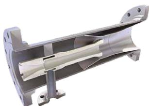
This type of desuperheater (known as a VTD) creates high velocity and turbulence to produce intimate contact between steam and cooling water to maximize the evaporation of water droplets. Pressurized cooling water enters the VTD through the cooling water branch; it then passes from the annulus through a series of small holes into the internal diffuser.
