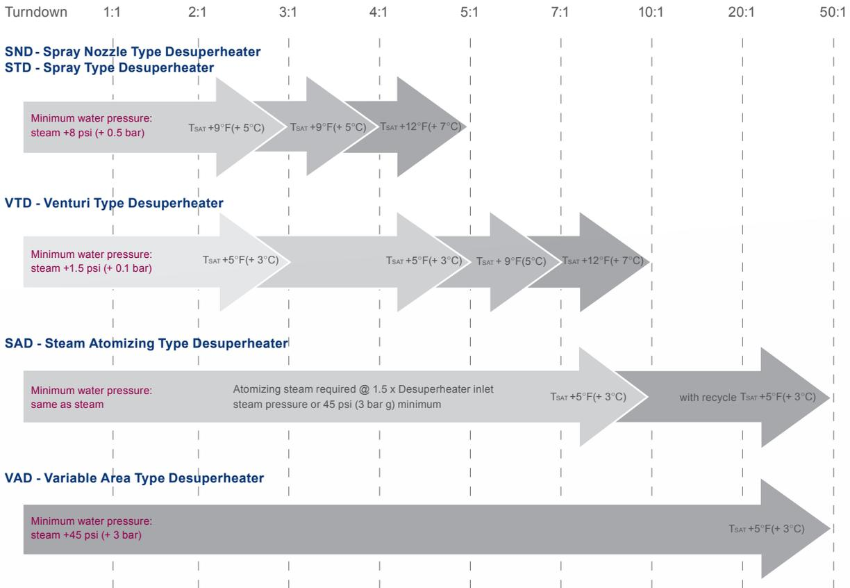
Turndown ratio is dependent on a wide variety of factors, such as installation (horizontal or vertical), amount of residual superheat, and piping. Dependant on conditions the turndown figures quoted for desuperheaters are the maximum capable.
