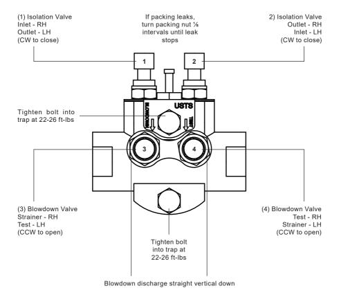
All valves use 1/2" socket, box, open-end or adjustable wrench
