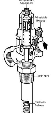
Remove the thread protectors from the valve and connect the piping without straining the valve body. Wrenches should be applied only to the hexagonal parts of the regulator—never on the valve body.
