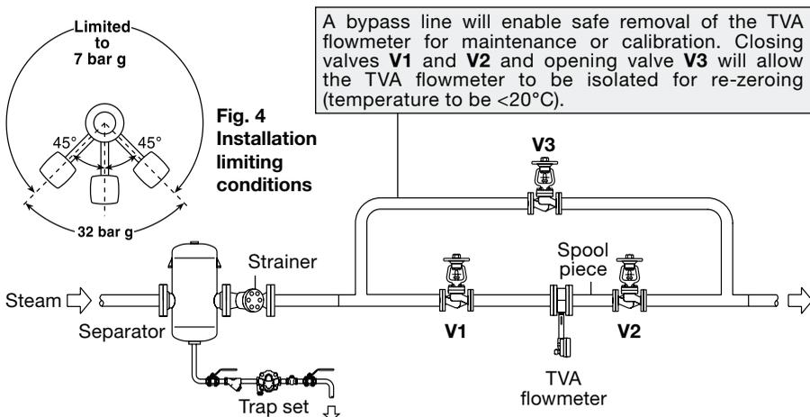
**Fig. 5 Typical installation**
