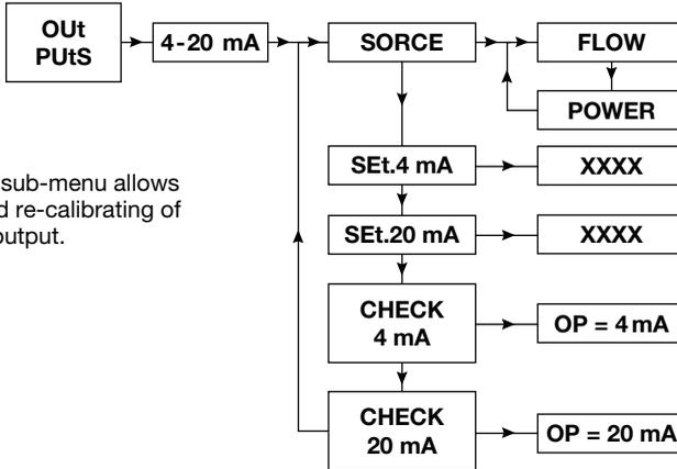
The 4-20 mA sub-menu allows re-ranging and re-calibrating of the 4-20 mA output.
