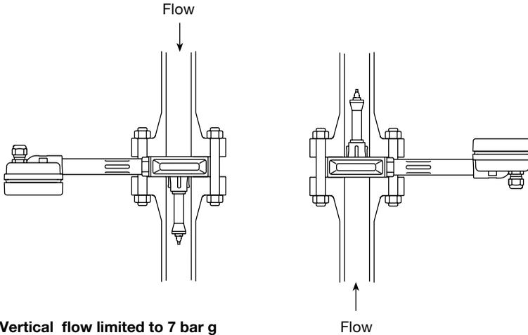
**Fig. 7 Vertical flow limited to 7 bar g**
