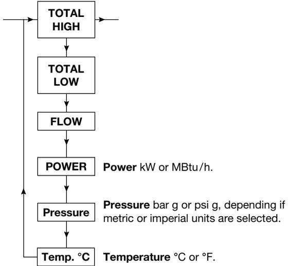
The following chart indicates the run mode data display sequence. Depending on the configuration, the flow units will be:
