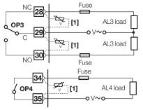
▲ The relay output OP1, OP2, can be used as alarm outputs only if they are not used as control outputs.
