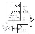
▲ In case of ON-OFF control, the LBA alarm is not active.
