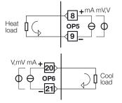
OP5 and OP6 outputs can be configured for control action or PV/SP/MV retransmission:
