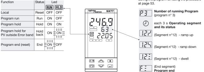
On program run mode, each 3 s the display shows alternatively:
