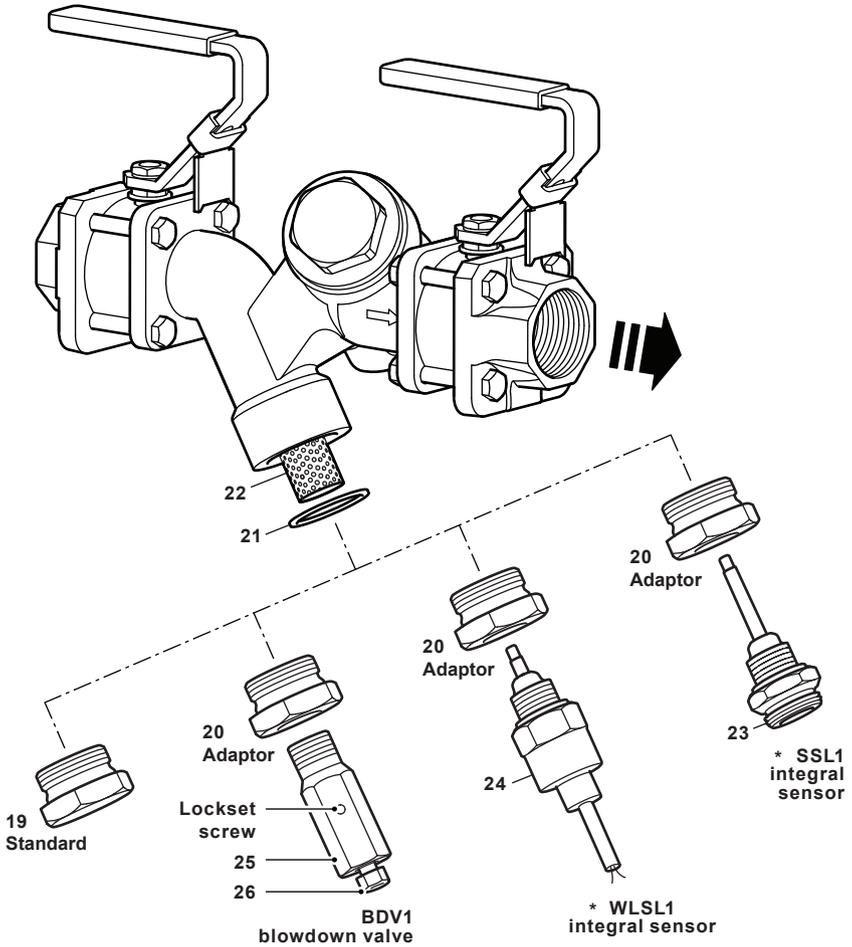
\* Please note that the optional Spiratec SSL1 and WLSL1 sensors (items 20 + 23 or 24) must not be fitted when the STS17.2 is installed in a vertical application.
