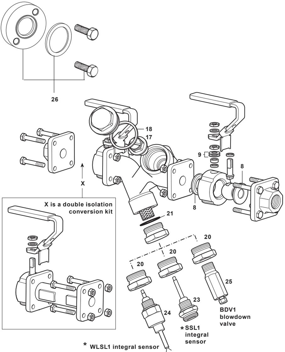
\* Please note that the optional Spiraxtec SSL1 and WLSL1 sensors (items 20 + 23 or 24) must not be fitted when the STS17.2 is installed in a vertical application.
