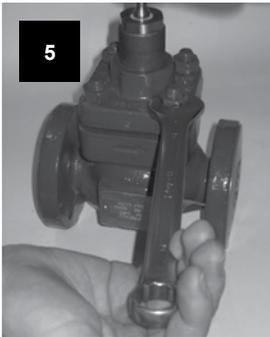
Using a torque wrench lightly and evenly tighten each bolt or nut by 45°, following the sequence illustrated in Figure 4, page 15.
