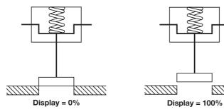
Fig. 33 2-port valve normally closed - TRAVL setting = 0 to 100%
