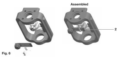
**5.2.2** Slide the bracket (2) to the left or to the right (Figure 6) till the correct position is achieved. If you're using a Spirax Sarco actuator the correct position is impressed on the magnet bracket (Figure 7).
