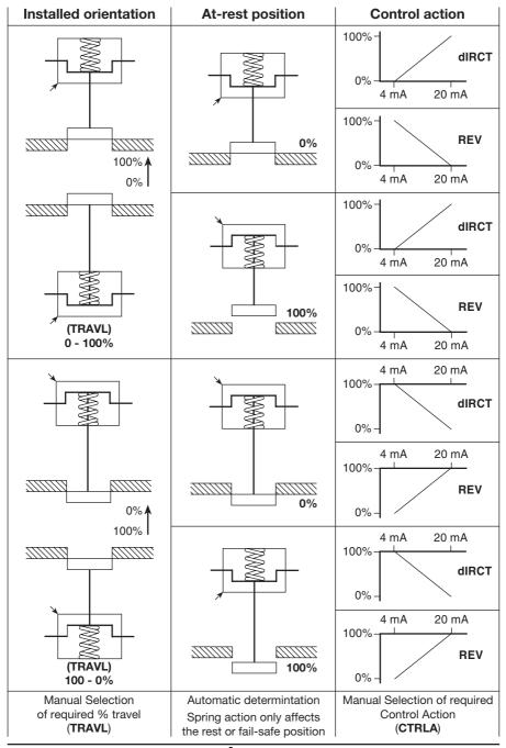
Fig. 42 CTRL Control Action dIRCT or REV setting guidance
