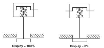
Fig. 36 2-port valve normally closed - TRAVL setting = 100% to 0%
