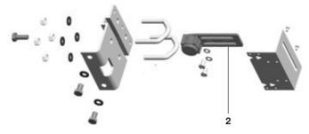
Fig. 4 Pillar mounting kit for a linear actuator
