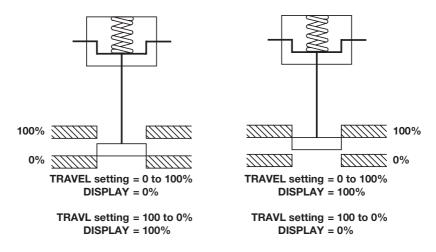
Fig. 37 3-port valve and spring extend actuator
