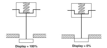
Fig. 35 2-port valve normally open - TRAVL setting = 100% to 0%
