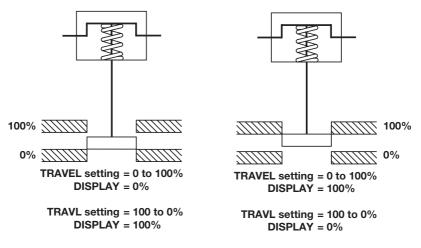
Fig. 38 3-port valve and spring retract actuator
