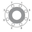
Flange bolts should be gradually tightened across diameters to ensure even load and alignment.
