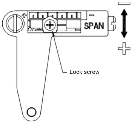
Fig. 23 Rotary span unit
