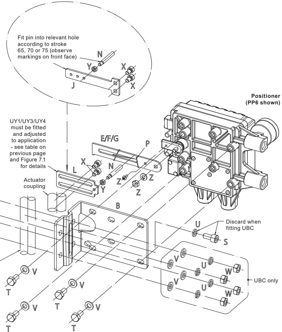
Fig. 7.2 Exploded view of side mount assembly (PP6 positioner shown)
