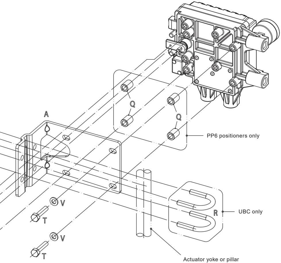
— Fit pin into relevant hole according to stroke 20, 30, 50 or 70 mm (observe markings on front face)
