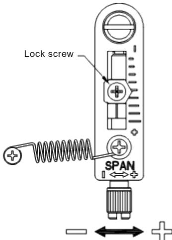
Fig. 22 Linear span unit
