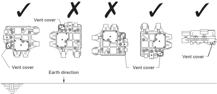
**Fig. 4** The correct positions of a vent cover
