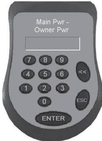
To exit the password input keypad, touch the ESC button which will return you to the “Welcome” screen (Fig.3).
