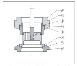
Figure 5 - Bellows Seal Bonnet with Seal
