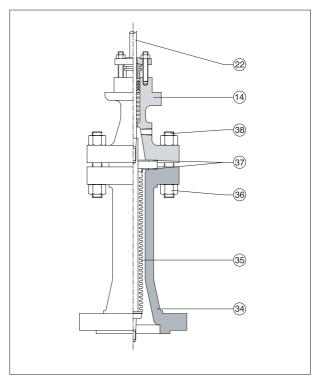
Figure 5 - Bonnet with bellows seal
