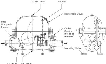
Inlet Baffle 3/4" NPT Plug (not to be removed)
