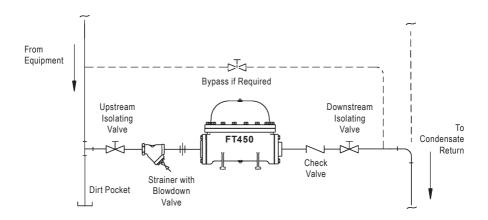
Before installing the trap, the inlet piping should be carefully blown down to remove any existing pipe debris.
