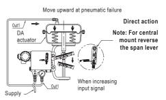
2.1.2 Piping and span direction setting for linear RA single actuator
