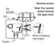
2.1.3 Piping and cam direction setting for rotary single actuator
