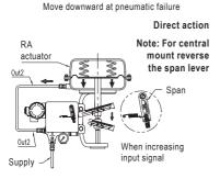
Move downward at pneumatic failure
