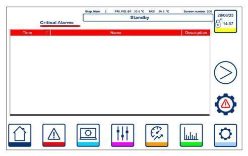
The notifications displayed on the Critical Alarms screen (200) are displayed to inform of the package not running within specification.
