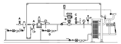
Fig. 6 The position of the pressure reducing valve in relation to other control equipment
