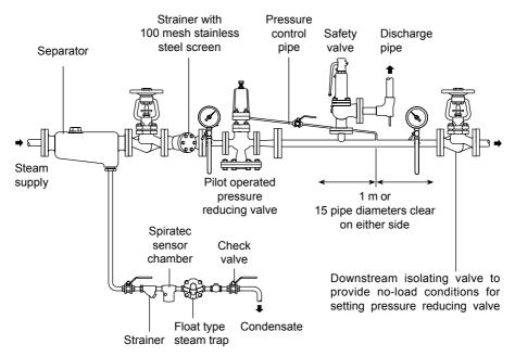
Fig. 2 Recommended installation
