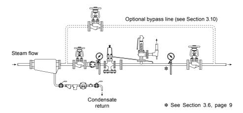
Fig. 4 Setting procedure sequence DP143, DP143G and DP143H
