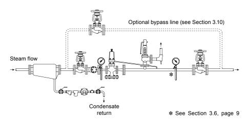
Fig. 5 Setting procedure sequence DP163, DP163G and DP163Y
