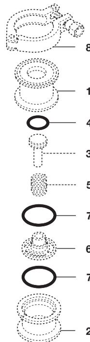
**Fig. 4 CVS10-1E with soft seat and sanitary clamp**
