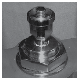
Fig. 18 Incorrect - thread protruding above the adaptor
