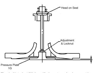
Fig. 4 Note in 1/2" thru 4" sizes, top of valve must be completely assembled and head must be on seat when measuring dimension "A" and when reassembling diaphragms.
