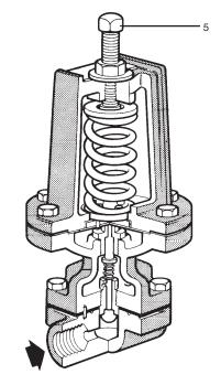
my be necessary to make a pressure readjustment. Repeat procedure 4 if required. Replace spring cover, then tighten adjustment locknut.
