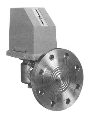
On request series 5500 can be equipped with oil filled **diaphragm separators** with capillary tube. This execution is suggested for measures where corrosive fluids or liquids with suspended matter are involved; particularly advisable for food applications.
