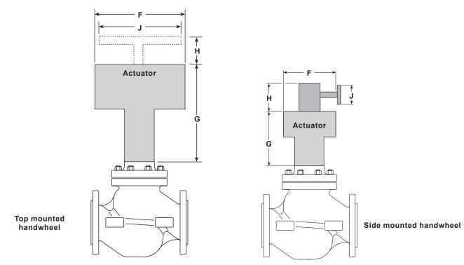
Dimensions/weights for the EL and AEL actuator ranges approximate in mm and kgs (and in inches and lbs)
