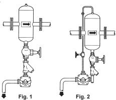
Note: with low condensate flow and CA14 air trap a compact installation and no balancing pipe are accepted (Fig. 1); for higher flow, a CA44 air trap and a balancing connection are required (Fig. 2).
