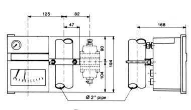
The mounting support can be of extended type allowing also the air regulator clamping.
