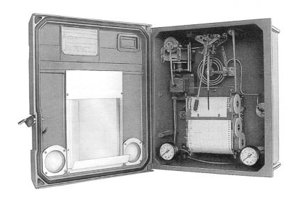
Example: Model 3689-T5C3-P2C2 - Two pens recording controller: for temperature measured with cylindrical bulb and capillary, gas filled thermometer system, suffix T5 (PI mode) and for pressure measured with Bourdon tube, suffix P2 (P model): Model 3682-P2C2-FS3 - Two pens recording controller: for pressure measured with Bourdon tube (P mode) and for flow rate measured with a pneumatic receiver, suffix S3 (recored only).
