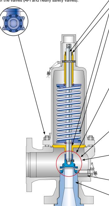
One piece spindle allows better alignment.
