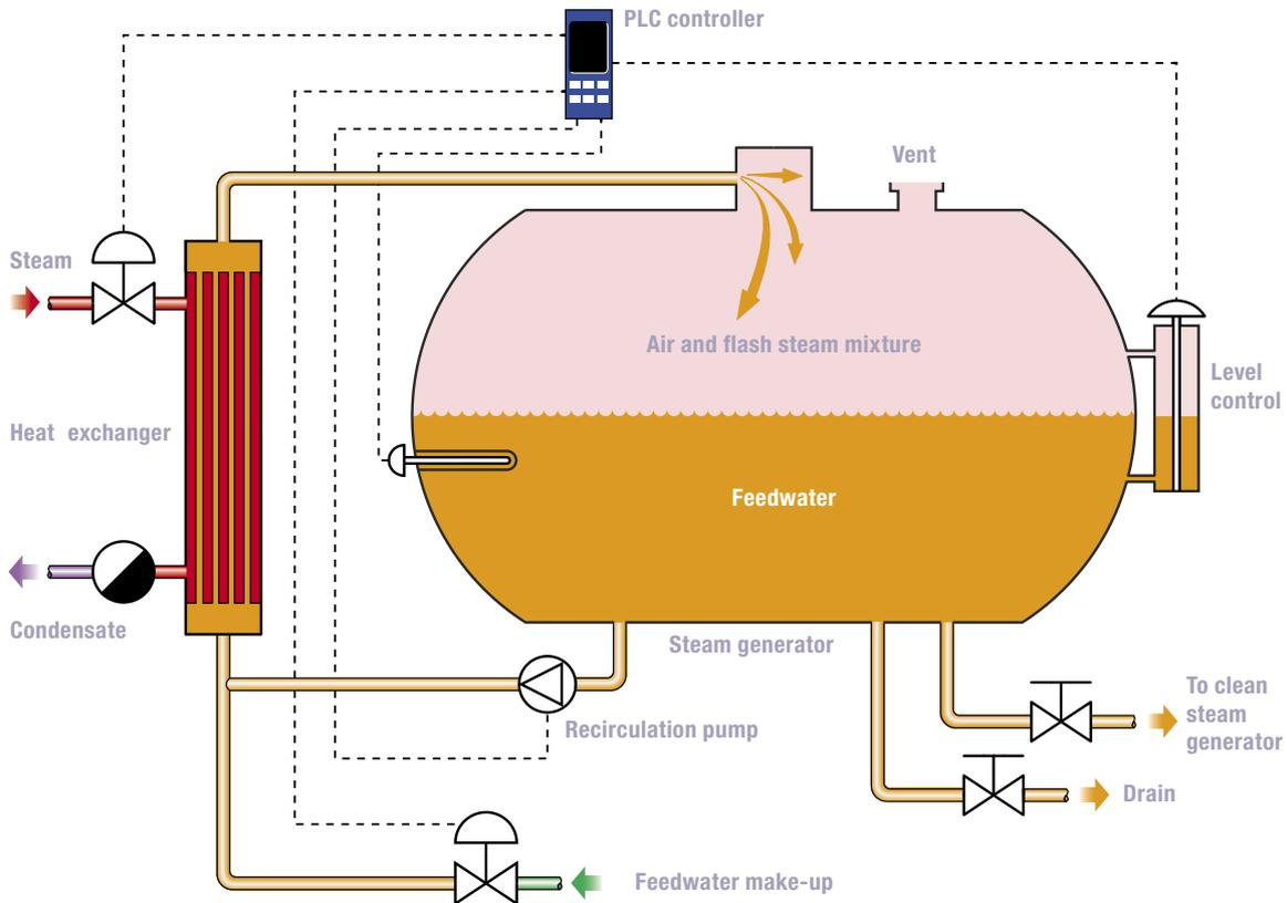
The treated water is recirculated through a primary steam heat exchanger to drive off non-condensable gases.
