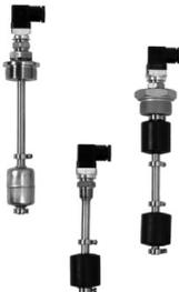
Compact type, recommended for applications in hydraulic control units. It can also be used with liquids with low specific weight such as hydrocarbons and mineral oils. Stainless steel or BUNAN floats, the other wetted parts are made of stainless steel. Can be equipped with reed switch contacts, allowing control of up to two switching points with a single instrument. In place of the housing, a three-pin DIN connector with flying plug is used.
