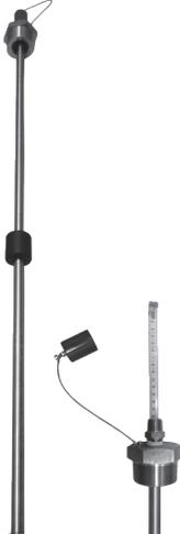
M Model is designed for applications on tanks that are not provided with level gauge and which requires manual and visual reading of the level. The level reading is achieved using a scale tape inserted into the rod: slowly pulling out the tape, it is possible to detect the liquid level through the interaction of the magnet of the float and the magnet on the bottom of the graduated tape. Floats are built in stainless steel or BUNA N, other wetted parts built in stainless steel.
