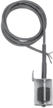
Type S is designed for applications in naval bilges to control oily and saline wastewater. It is also serviceable in hardly accessible compartments, where it is necessary to detect the presence of liquids. Fittings with reed switch contacts, SPDT or 1 DPDT, to control a single switching point. TOR S is not equipped with housing. A sheath of heat-shrinkable material protects the NFO output cable. The enclosure rating is IP68
