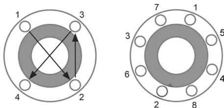
Flange bolts should be gradually tightened across diameters to ensure even load and alignment.
