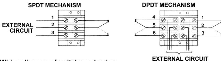
Fig. 3 - Wiring diagram of switch mechanism
