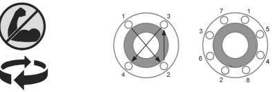
Do not over tighten. Use correct torque figures.
