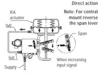
Move downward at pneumatic failure
