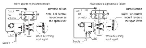
2.1.2 Piping and span direction setting for linear RA single actuator
