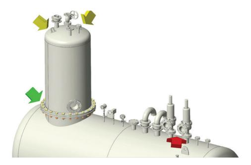
Lift the deaerator head using a crane or appropriate authorised handling system (yellow arrows), then attach the head to the tank nozzle using tie bolts (green arrow).
