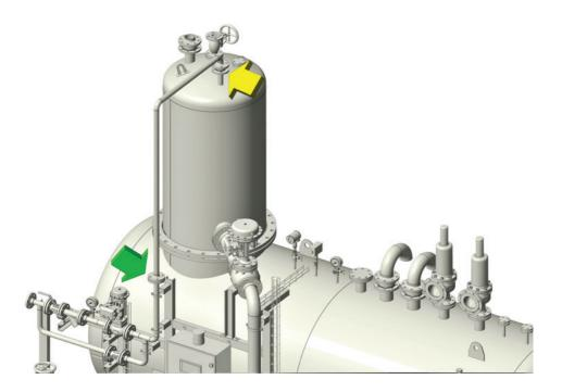
Fasten the make-up water inlet spool (yellow arrow) to the deaerator head nozzle and then fasten it to the outlet spool, already fastened to the frame (green arrow).
