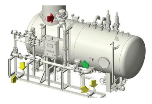
Lift the steam injection and water inlet assembly skid using the four lifting eyebolts (yellow arrow) welded to the support frame using a crane or adequate authorised handling system.
